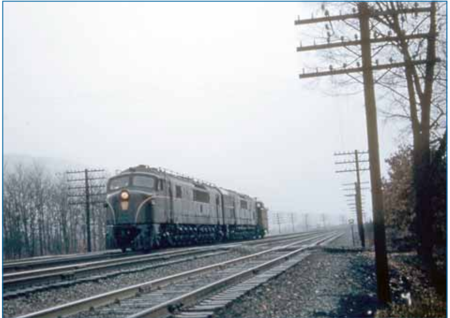
Above is the most monstrous of PRR diesel classes, the "centipede". They began life as passenger units, but were quickly downgraded not only to freight units but w/"helper" designation (1st class BP60, 2nd class BH50 - lost some HP in regearing). Here are a pair clunking along on main line east of Altoona in 1959. They only last a couple more years. - submitted by Fred Ripley, Murray, KY
